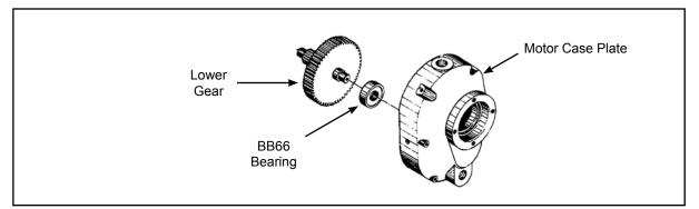
• Press the upper gear bearing (525424) and lower gear bearing (BB66) into the gear case.
