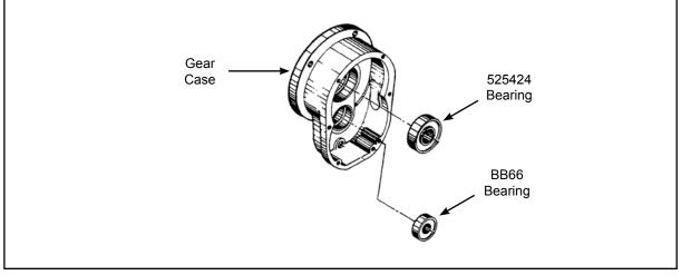
• Position the gasket on the motor case plate and assemble the gear case.
