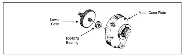
• Press the upper gear bearing (BB124) and lower gear bearing (1004572) into the gear case.
