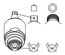
→ To avoid air pockets, fill the filling hole full of oil.
