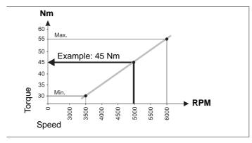
Settings example: Tightening: 45 Nm Screw M10: 8.8
