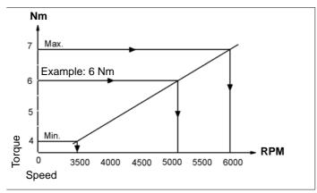
Settings example: Tightening: 6 Nm Screw M5: 8.8
