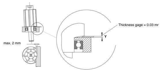
2. Examine Y with thickness gage. If dimension > Y, step 1 with support <C5>, <C6>, <C7> repeat.
